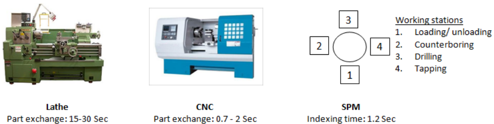
Fig. 17. Part exchange time on traditional lathe, CNC, and SPM.
